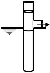
**The outlet T-joint** is installed to retain the scum layer within the tank.
