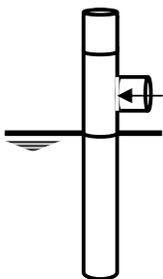
**The inlet T-joint** dissipates the energy of the incoming flow and deflects it downwards. *The vertical leg of the tee extends below the liquid surface well into the clear space below the scum layer.* This prevents disturbance of the floating scum layer and reduces disruptive turbulence caused by incoming flows. The inlet T-joint device also prevents short-circuiting of flows across the water surface directly to the outlet.
