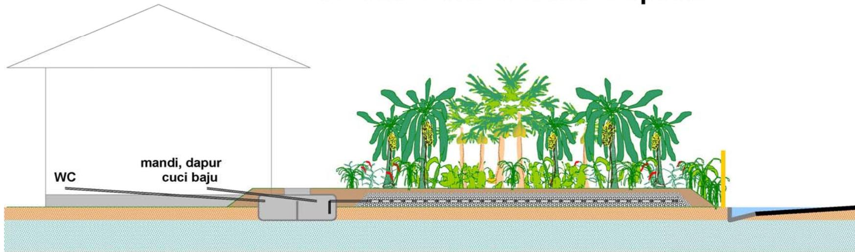
Leachfield and septic tank are covered with a layer of soil
